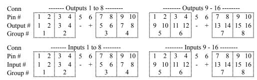
Voltage applied to pin 6 of the two output connectors can be changed by the position of the shorting bar. The standard position provides 5 volts when the SRC162 is driving LEDs or other low current 5 volt devices. See section 5.3.
