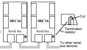
In a systems when more than 10 SRC162s are used the bus terminating resistor should be cut on any additional devices.
