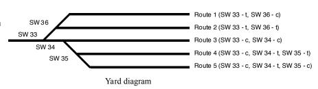
A route can be executed with an actual turnout (switch) address or a pseudo address of a switch (not a physical switch). Program the top address of the route with the address you want to execute the route. Inputs can be programmed to execute a route from a push button.
